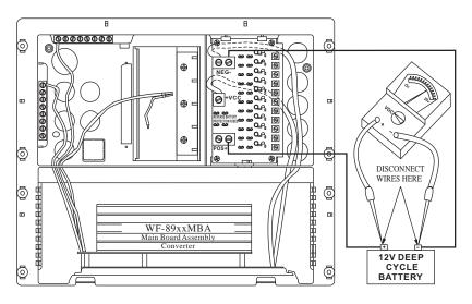
If the converter output voltage at the battery reads in the 0.0 Vdc range, or the battery is not charging, check for:
